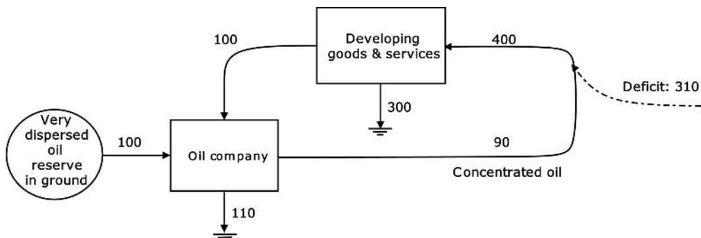
Figure 19 Example of oil reserve which cannot sustain its own extraction and refining
