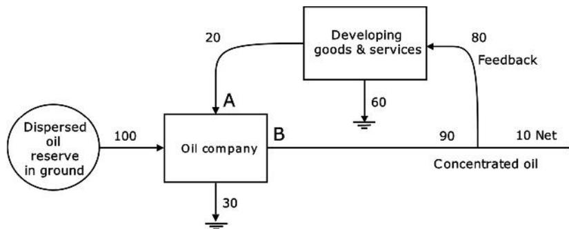
Figure 18 Example of oil reserve near the end of its life
