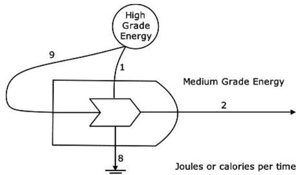
Figure 16 Wasteful use of high-quality energy to produce medium-quality energy
